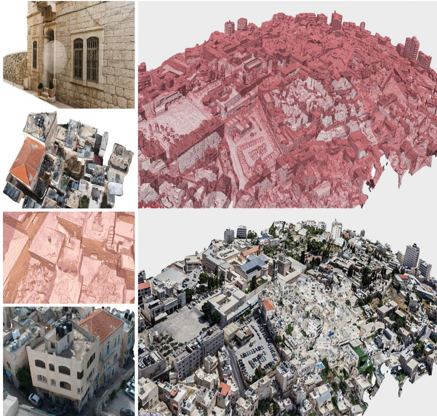
Fig. 4. Output of photogrammetric survey Structure from Motion (SfM), terrestrial and aerial UAV, integrated to guarantee a global and complete coverage of urban environments and volumes
