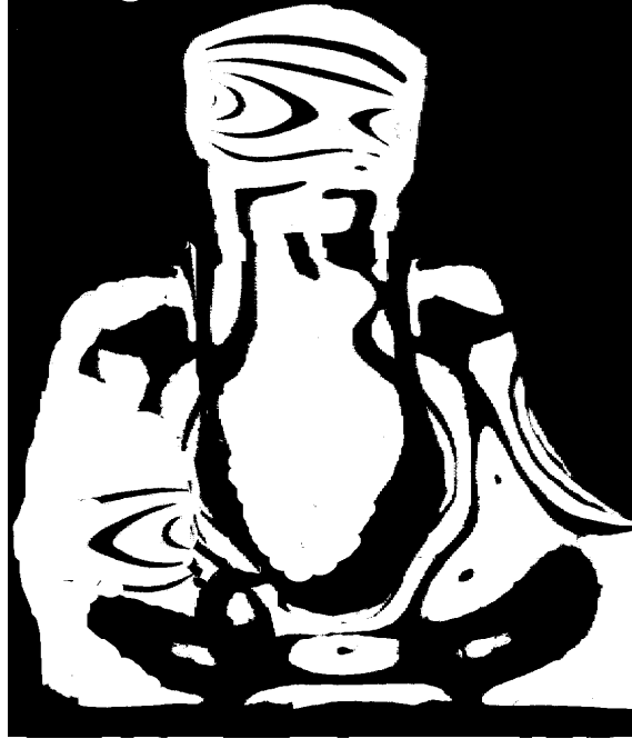
Fig 8 The fringe pattern in the teeth-jaw model under luxation.
