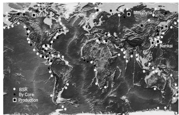
Fig. 9. Continental and subaqueous manifestations of gases and hydrates: BSR – supposed gas hydrate deposits; by core – confirmed gas hydrate deposits; production – gas hydrate deposits under development; Mallik – gas field in the delta. Mackenzie, Canada; Messoyha – gas hydrate deposit located in the north-east of Western Siberia, 250 km west of the city of Norilsk; Nankai – gas hydrate field on the shelf of Japan in the region of the eastern Nankai trough
