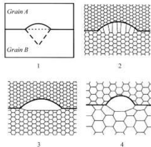
Fig. 6. Schematic representation of nuclei formation according to SIBM mechanism [49]
