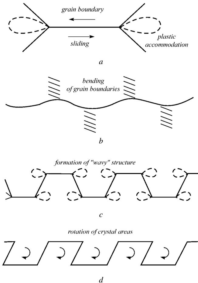
Fig. 8. Schematic representation of formation of recrystallized grains [67]; a) process of grain boundary sliding, leading to increased stresses near triple junctions; b) bending of grain boundaries caused by boundary migration; c) grain boundary sliding in some areas of the boundary and dislocation sliding, leading to "wavy" structure formation; d) dislocation sliding in elongated areas, leading to rotation of small areas
