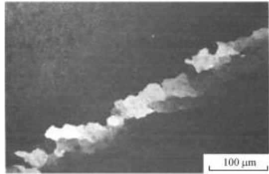
Fig. 7. "Core and mantle" structure in the boundary resulted from aluminium polycrystal deformation (Al-5%Mg), the strain is 0.6, the temperature is 723 K, the strain rate is  $2 \cdot 10^{-3}$  s $^{-1}$  [67]
