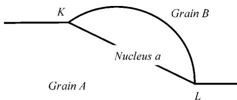
Fig. 2. Schematic representation of formation of nucleus *a* by bending the ledge *KL* from grain *A* to grain *B* with higher stored energy [59]
