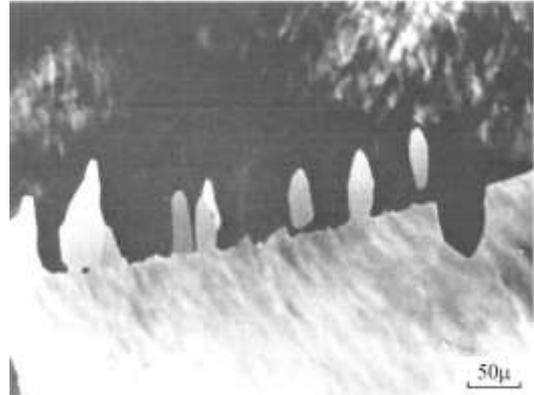
Fig. 5. Nuclei formation of new grains according to SIBM mechanism in aluminium polycrystal which had been deformed by 40 % and annealed during 1 hour [49]
