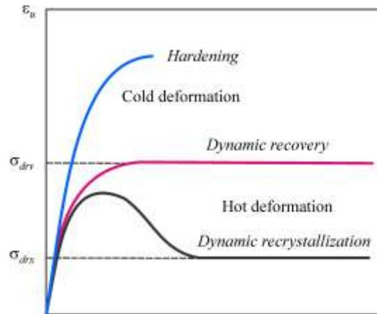
Fig. 9. Typical " $\sigma$ – $\epsilon$ " is the loading diagram for metals under different temperatures and processes of a high-temperature deformation;  $\sigma_{drv}$  are characteristic stresses of dynamic recovery,  $\sigma_{drc}$  are characteristic stresses of dynamic recrystallization
