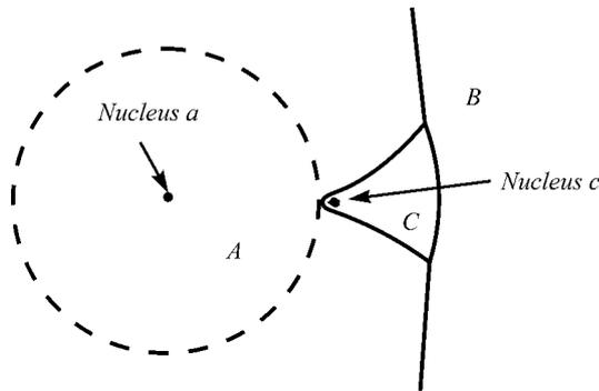
Fig. 1. Schematic representation of nuclei formation and growth [54]; *a*, *c*: nuclei of new grains; *A*, *C*: grains subjected to recrystallization; *B*: original grain of polycrystal
