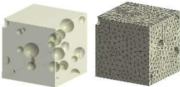
Fig. 9. Model (transparent) and finite element mesh for porosity of 6 %
