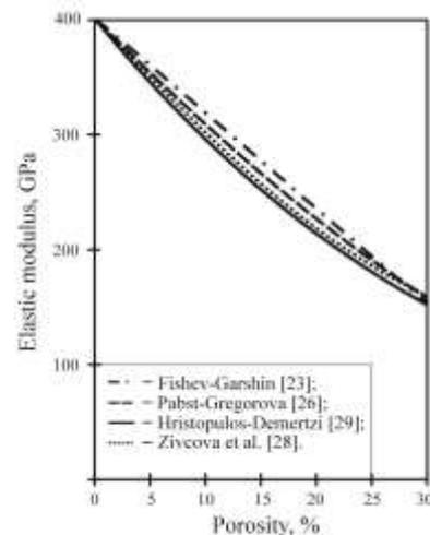
Fig. 2. Relations describing the change of the elastic modulus  $\alpha\text{-Al}_2\text{O}_3$  for different porosity
