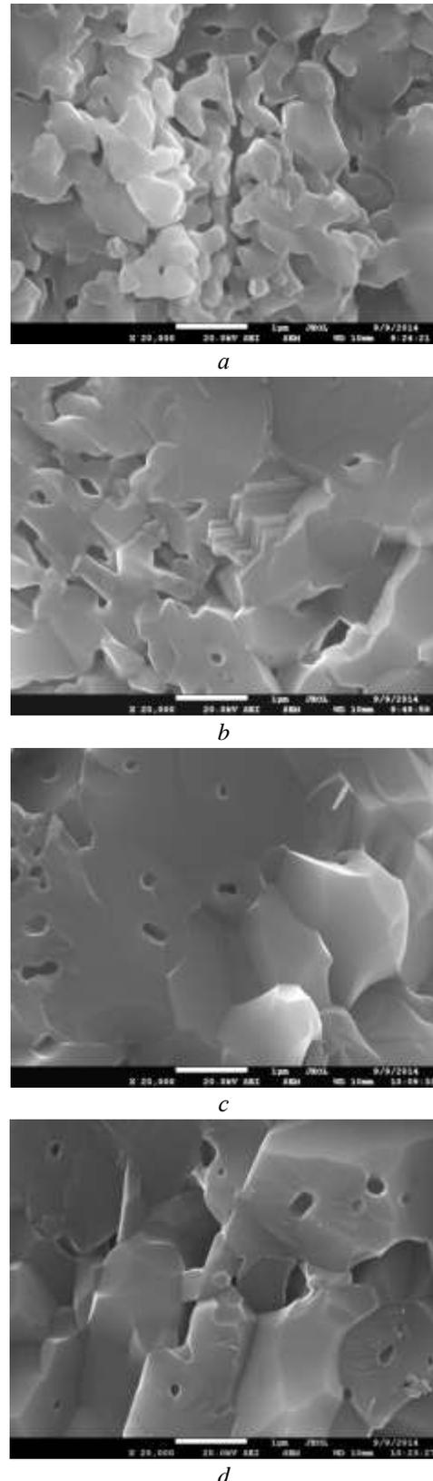
Fig. 7. The surface of the break in ceramic specimens with different porosities (a – 0.24; b – 0.11; c – 0.06; d – 0.04)
