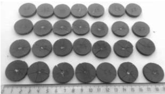
Fig. 4. The specimens after testing according to the scheme of the Piston-on-Ring bending test
