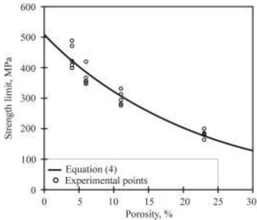
Fig. 6. The dependence of the material ultimate strength of ceramic specimens on porosity
