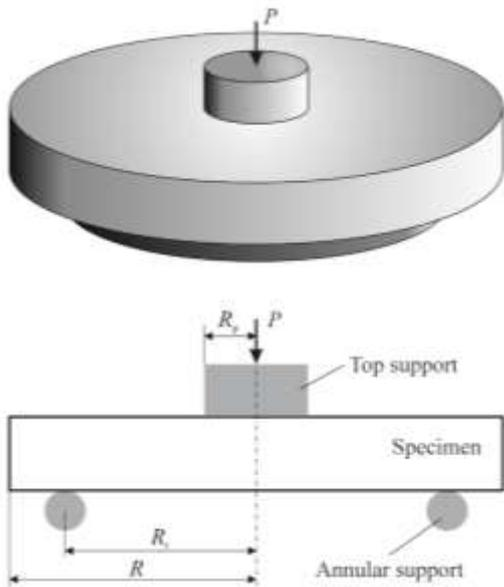
Fig. 3. The scheme of the specimen on a ring support
