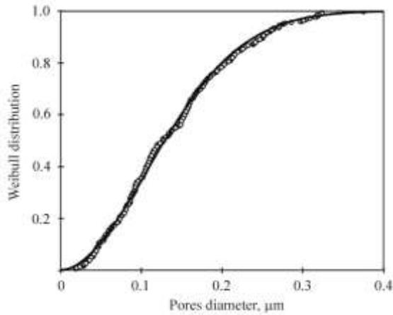
Fig. 8. Weibull distribution of pores diameter
