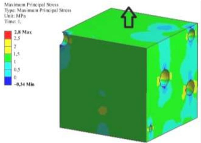
Fig. 10. Distribution of first principal stresses in the cell under uniaxial tension (the porosity of 6 %)
