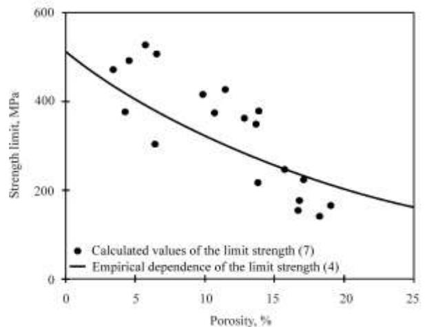
Fig. 11. The dependence of the material ultimate strength of ceramic specimens on porosity
