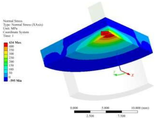
Fig. 5. Distribution of first principal stresses across the width of the specimen with the porosity of 4 %
