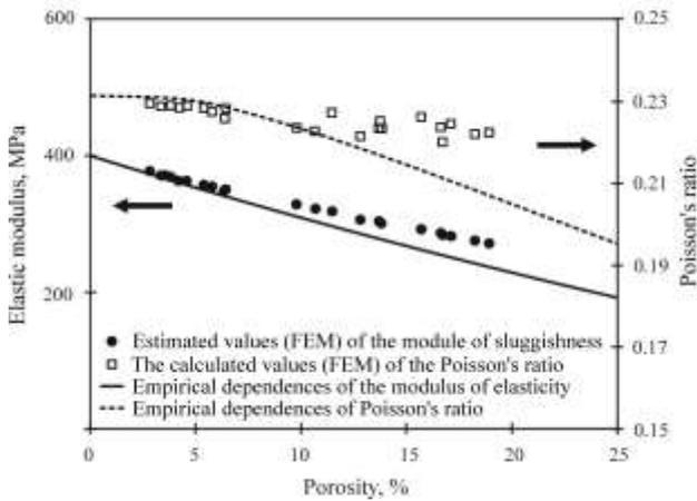
Fig. 12. The dependences of the elastic modulus and Poisson's ratio for ceramics on porosity
