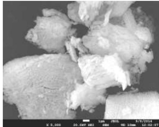
Fig. 1. The initial powder  $\text{Al}_2\text{O}_3$  (agglomerates)
