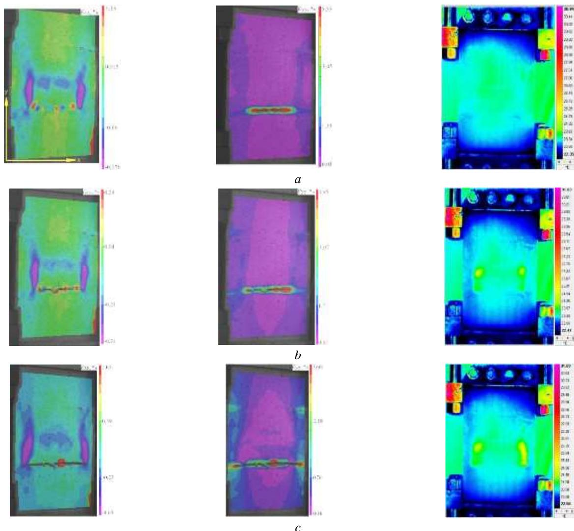
Fig. 8. Deformation fields  $\epsilon_{xx}$ ,  $\epsilon_{yy}$  and thermal images on the specimen's surface in the course of tension under static load testing after preliminary cyclic loadings: *a* – corresponds to point 1 of the diagram; *b* – corresponds to the point 2; *c* – corresponds to point 3
