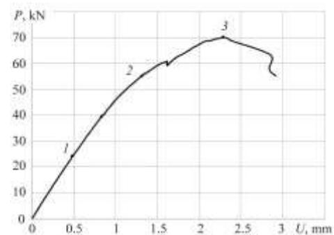
Fig. 7. The loading diagram of the ASP specimen under tensile test after preliminary cyclic effects
