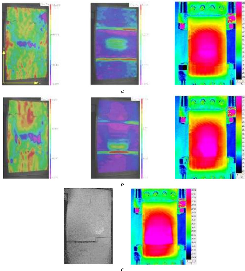
Fig. 4. Deformation fields  $\epsilon_{xx}$ ,  $\epsilon_{yy}$  and thermal images on the specimen's surface during the static tension test (a, b), the image and the thermogram at the moment of fracture (c): a – corresponds to point 1 of the diagram; b – corresponds to point 2; c – corresponds to point 3
