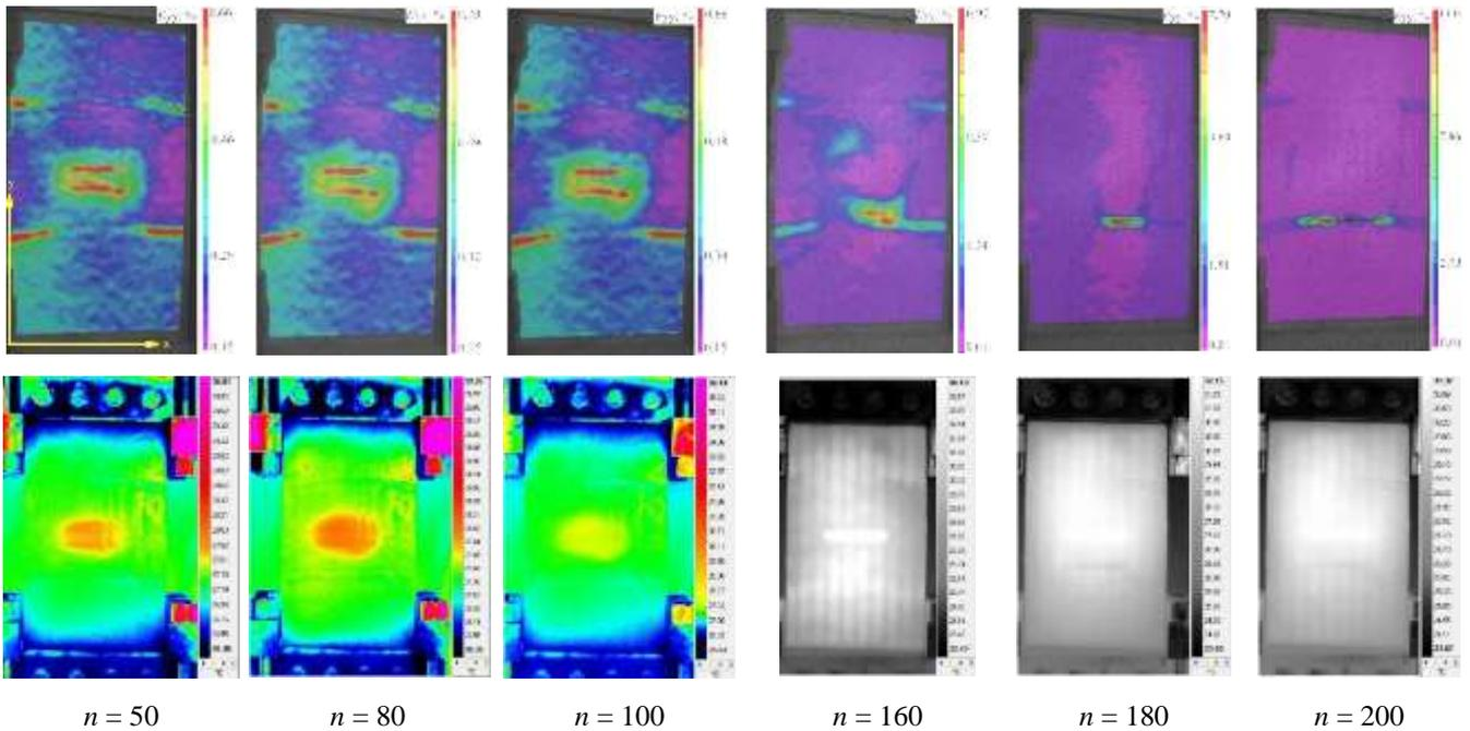
Fig. 5. The evolution of the longitudinal deformations (at the top) and corresponding thermal images (at the bottom), depending on the number of the implemented loading cycles
