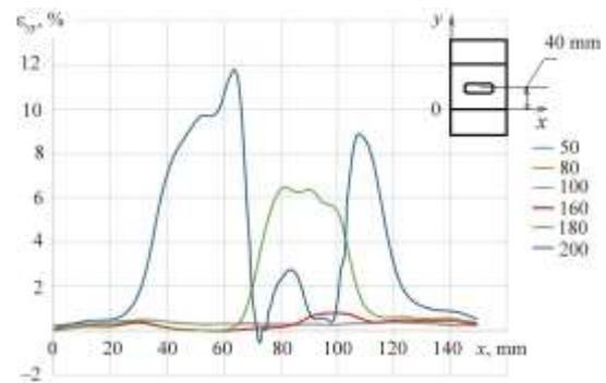
Fig. 6. Diagrams of the longitudinal strain distribution  $\epsilon_{yy}$  along the line of the bottom repair zone across the whole width of the ASP specimen under cyclic tests, corresponding to the inspection points of registration, when reaching 50th, 80th, 100th, 160th, 180th and 200th loading cycles
