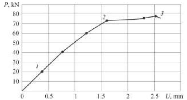
Fig. 3. Loading diagram of the ASP specimen under tensile test
