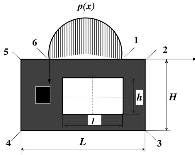
Fig. 2. Mezoelement of porous sheeting.
