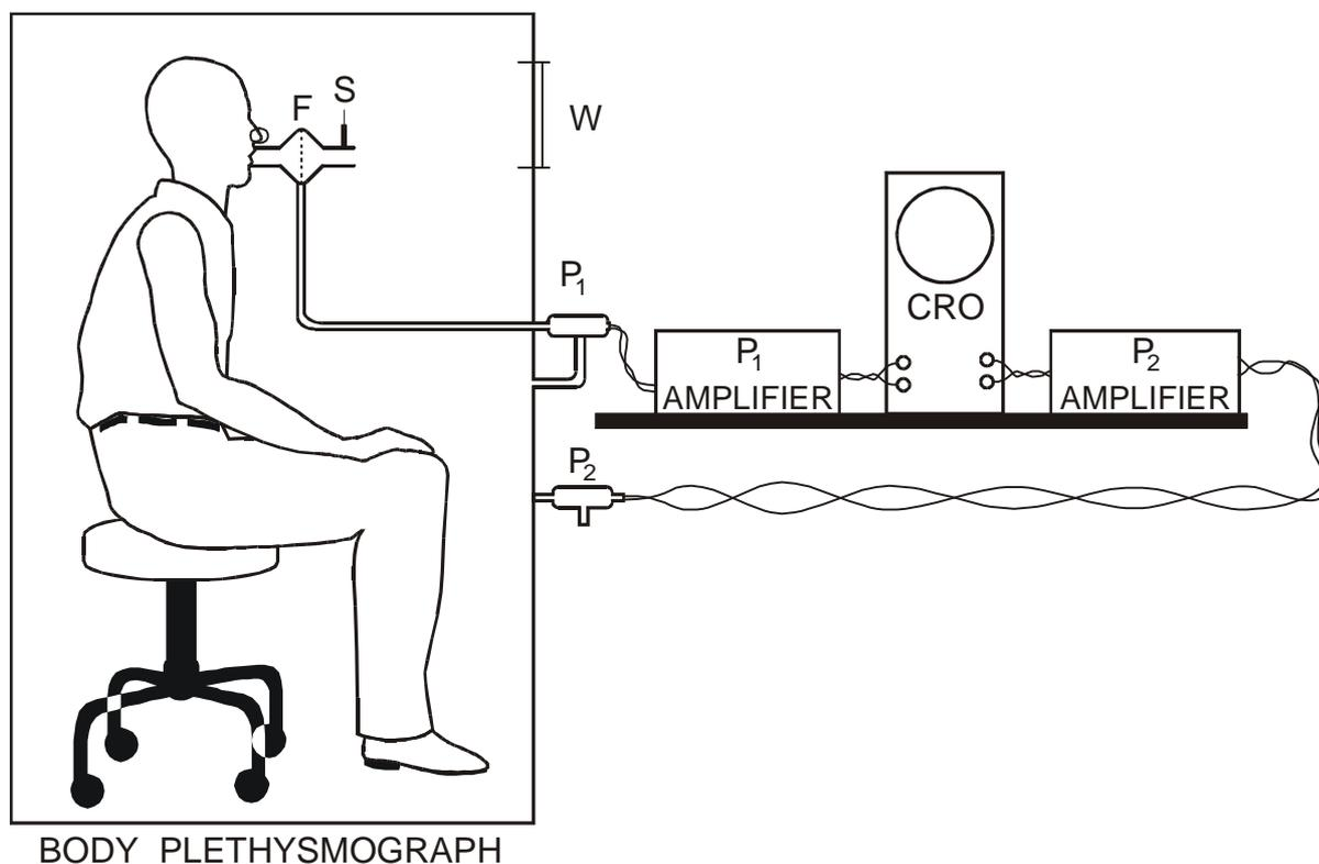
Fig. 2 The apparatus for measuring the respiratory tracts resistance. CRO - cathode-ray oscilloscope.
