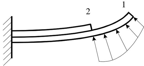
Fig. 5. The scheme of the joint bending of two curved plates.
