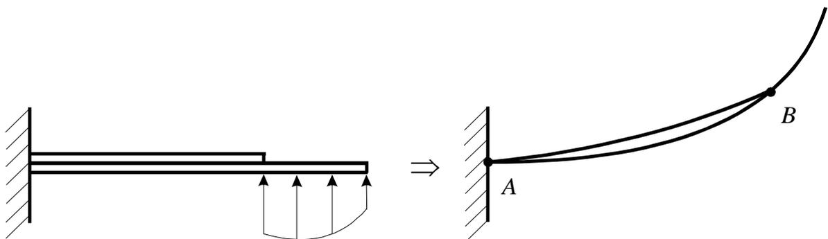
Fig. 1. The contact of the plates takes place at the points  $A$  and  $B$ .
